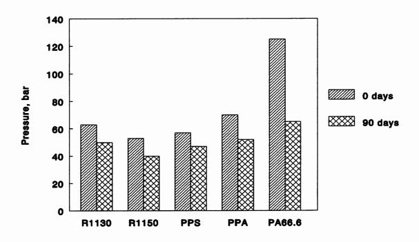
Figure 2: Static burst pressure measured before and after ageing in 90°C water for 90 days
