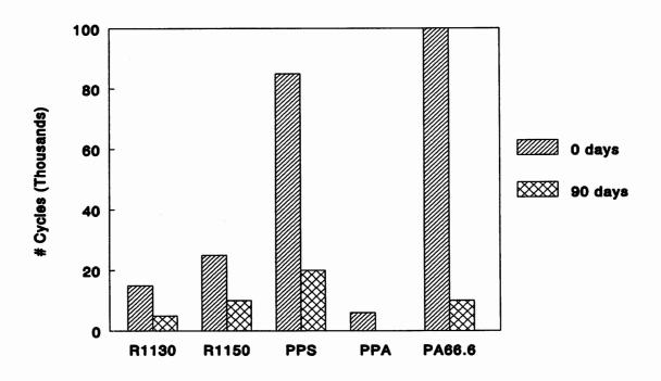
Figure 3: Dynamic burst pressure measured before and after ageing in 90°C water for 90 days
